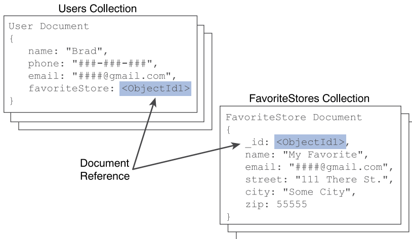
Figure 11.1 Defining normalized MongoDB documents by adding a reference to documents in another collection
