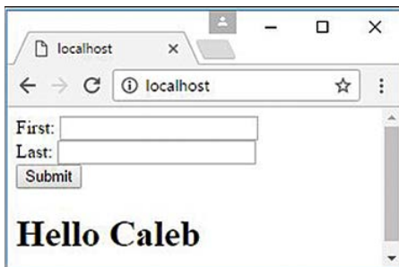
Figure 19.2 Handling POST parameters in the request body using the bodyParser middleware
